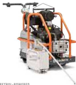
PETROL-POWERED HUSQVARNA SOFF-CUT 4000 Diamond blade max 350 mm, cutting depth max 70 mm, 191 kg, 14.9kW*.
