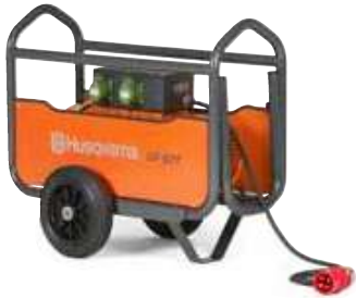
ELECTRIC-POWERED HUSQVARNA CF 67T Output 42 V–3–200 Hz, 4.7 kVA, 67 A, 70 kg, 4 outlets.
