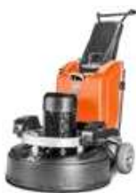
ELECTRIC-POWERED HUSQVARNA HTC 950 RX 15 kW, 380–415, 440–480 V, 3-phase, grinding width 920 mm, grinding disc 4 × 270 mm, 600 kg.
