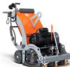
ELECTRIC-POWERED HUSQVARNA BMC 335 16 kW, 400V/32-63A, 335 mm working width, 430 kg.
