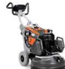
ELECTRIC-POWERED HUSQVARNA HTC 5 4.0–2.2 kW, 400–220 V, 3-phase/1-phase, grinding width 515 mm, grinding disc 3 × 230 mm, 122/179 kg.
