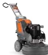
ELECTRIC-POWERED HUSQVARNA PG 830 RC 16.5 kW, 380–415 V, 3-phase, grinding width 800 mm, grinding disc 3 × 270 mm, 598 kg.
