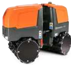
DIESEL-POWERED HUSQVARNA LP 9505 18kW, drum width 850mm, 1680kg.
