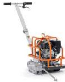
PETROL-POWERED HUSQVARNA SOFF-CUT 150 Diamond blade max 150 mm, cutting depth max 30 mm, 40 kg, 3.5kW*.
