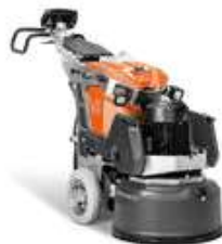
ELECTRIC-POWERED HUSQVARNA HTC X6 / HTC RX6 7.5 kW, 380–415 V, 3-phase, grinding width 600 mm, grinding disc 3 × 230/4 × 230 mm, 384/441 kg.
