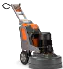
ELECTRIC-POWERED HUSQVARNA HTC 830 S 11 kW, 380–415 V, 3-phase, grinding width 800 mm, grinding disc 3 × 270 mm, 497 kg.
